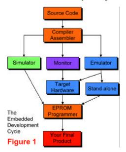
The debugged object code is re-compiled. For the final product the debug information is removed and a file is produced in a standard format such as Motorola Srecords. This file will be stored in the final product's nonvolatile memory such as EPROM or FLASH. This process is illustrated in Figure 1. This memory can be external or internal to the microcontroller. The HC11 has OTP (unerasable EPROM) and the HC12 has FLASH and EEPROM. ©2002 Nohau Corp Version 2.1 October 15, 2002
