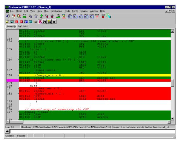
The Code-Coverage information can also be displayed in raw mode as seen below listing the address ranges of the instruction that have been executed and supplying a summary as seen below. This information is also available in a text file, to allow further processing outside the Seehau software if needed (further processing can also be achieved using Seehau's built in macro language).
