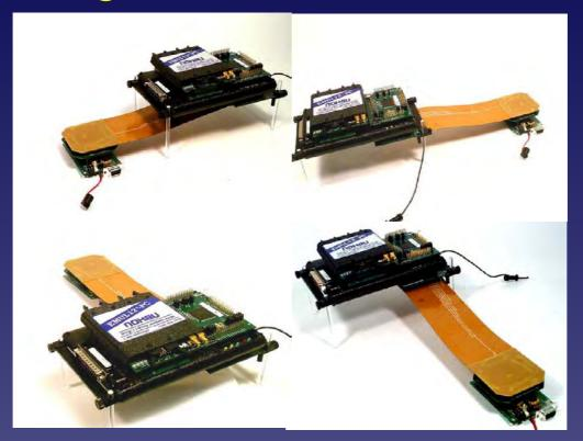
HCS12 Target Boards are often buried deep between modules, with very limited access to the HCS12 target board. The Nohau Flex-Cable resolves this problem by allowing to escape from the target, and connect to the full-emulator, in any of 4 directions. The flex-cable is also designed for high-speed operation above 100MHz, and includes controlled impedance and shielding
