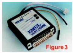
A BDM debugger does not have trace memory, triggers or emulation memory. A BDM emulator is sometimes used in conjunction with a full emulator. It is the preferred method used to program FLASH and EEPROM in the HC12 controller in your target system.
