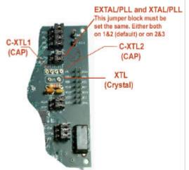
TRG-XTAL and making sure that the XTL, C-XTL1 and C-XTL2 pin sockets are un-populated. The default position for both of these jumpers is PLL. It is not recommended to drive the analog EXTAL and XTAL signals from the target as they will be susceptible to noise due to the long distance.
